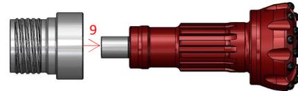
10. Fit the Bit Retaining Rings to the retaining area of the Bit shank.
