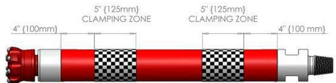
Position the break out bench chain clamps in the appropriate clamping zone positions to avoid damaging the hammer Wear Sleeve when breaking apart or assembling.
