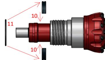
12. Thread the assembled Bit, Driver Sub and Bit Retaining Rings into the end of the Wear Sleeve.
