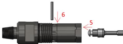
7. Insert the Piston into the assembled Top Sub.
