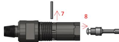
9. Pull the Check Valve away from the Spring in the Air Guide.
