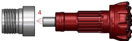
5. Unthread the Wear Sleeve, slide it over the Piston and away from the Top Sub.
